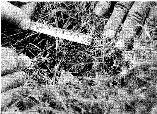
Fig. 2 Char fragment from SPTB motor firing.
